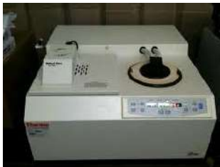
8. Concentrador-evaporador de muestras SPD1010 (Thermo Scientific).
